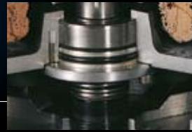
Heavy-duty, greased-for-life ball bearings. Double shaft seal system with intermediate oil chamber. SiC/SiC primary seal.
