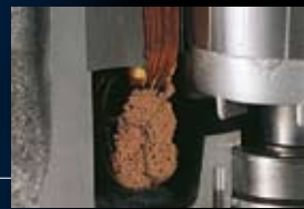
Stator is insulation class F (155 C). Built-in thermal switch for protection of the motor. The motor will stop before overheating can cause any damage to the system.
