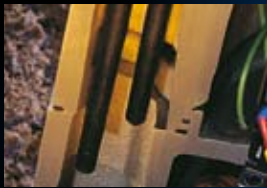
Electrodes for monitoring the water level in the water level compartment and automatic operation of the pump. 24 V control voltage. No moving parts for start and stop signal.
